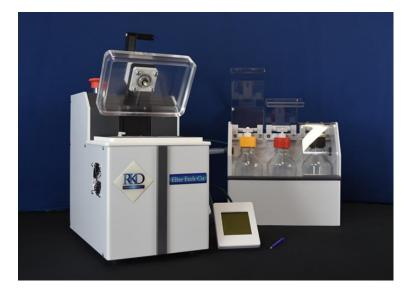
delivery rate allows decapsulation of copper wired devices with no wire or metallization damage. The specially designed acid heat exchanger can accurately control the acid temperature between 10° and 250° C with flow rates of up to 8 ml per minute. The high acid pulse rates allow for reasonable etch times even at the lowest temperatures.
