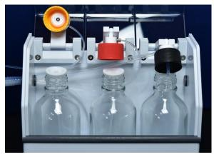
The **Elite Etch** is designed to fit comfortably inside of a fume hood while maintaining all necessary safety features. By using a heat exchange system, waste acid is cooled below 90 C to allow the use of a single waste bottle. The **Elite Etch** uses 3 standard 500 ml bottles which are supplied with the system.
